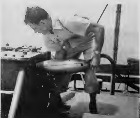
A TELEPHONE "pickup," attached to a cable, is eased overboard from the "recorder ship." The "pickup" will transmit the shock waves to the seismograph.
